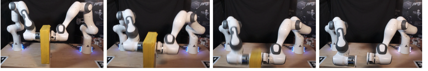
(a) Without motion adaptation, the box dropped when the arms were teleoperated to stretch forward and reached the shoulder joints' maximum torque limits.
