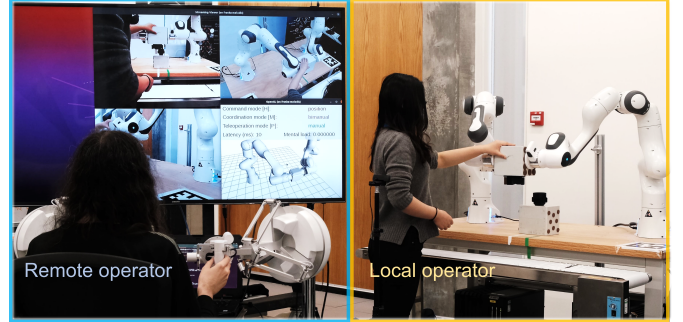
Fig. 1: Real-world part assembly task performed via teleoperation and direct physical interaction using the proposed collaborative bimanual manipulation framework.
