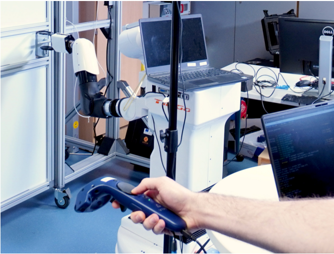
Fig. 5. INRIA TIAGo-2 teleoperated with the HTC Vive 6-DoFs pose controller to open the door.
