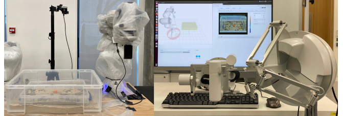
Fig. 1. Experimental setup: The replica robot is a Panda 7-DoF Manipulator Arm with mock terrestrial planet environment, and the master setup is a Sigma.7 with a GUI.
