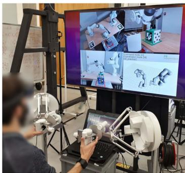
User interfaces for multi-contact teleoperation. *Left*: Operator commands free end-effectors' pose and triggers contact switch. *Right*: Remote bimanual docking and assembly task.
