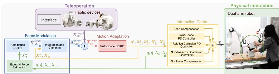
Overall architecture for bimanual manipulation of heavy object. Admittance controller generates velocity commands from external guidance forces on object. Velocity commands from interaction and absolute pose commands from remote operator are combined. SEIKO adapts combined commands to produce feasible desired posture and contact wrenches. Interaction controller realizes the desired configuration using passive impedance and load compensation.
