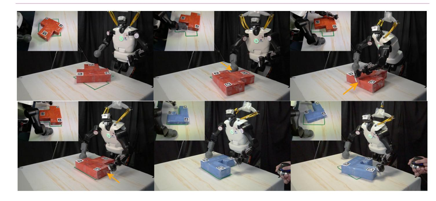
The robot uses both hands for non-prehensile manipulation, making and breaking contact
