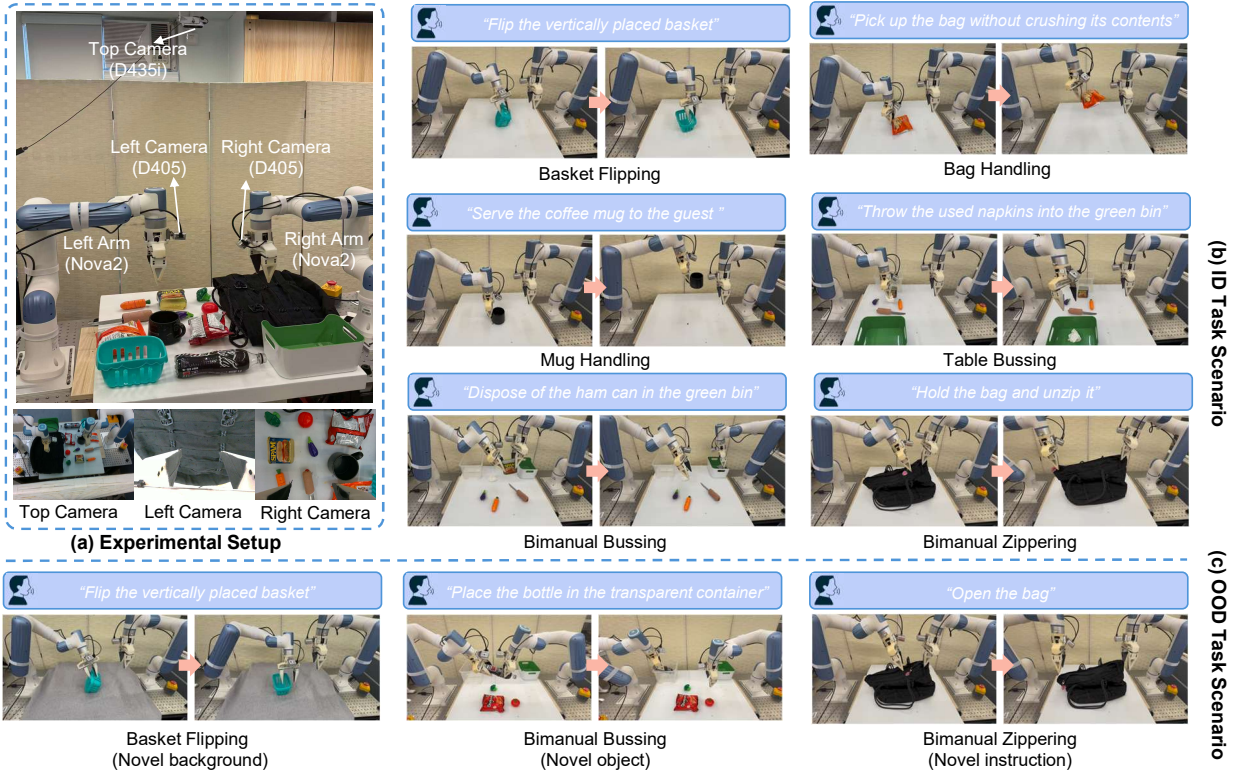
Fig. 5. Qualitative results of real robot experiments. VLA-Pilot effectively steers off-the-shelf pre-trained VLA policies to complete downstream tasks at inference time, achieving zero-shot deployment across both ID and OOD task scenarios.
